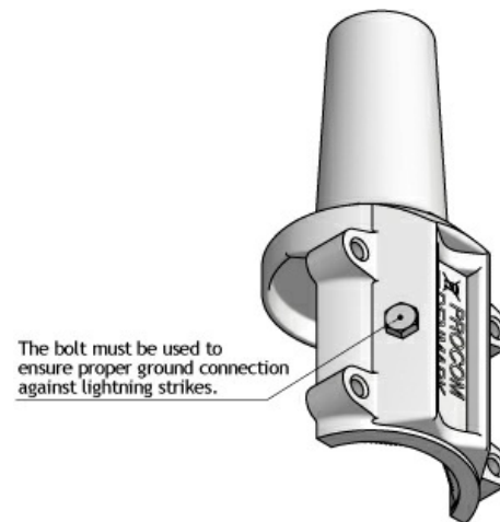
MOUNTING DESCRIPTION FOR GROUND CONNECTION
