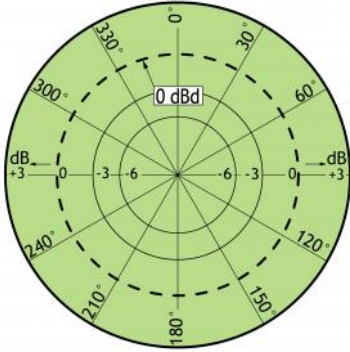
TYPICAL RADIATION PATTERN (H-PLANE)
