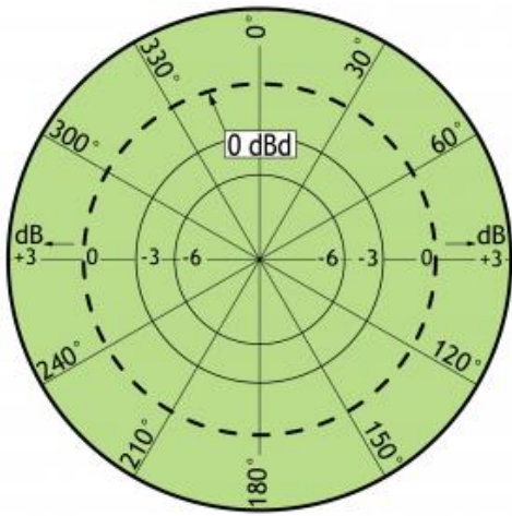
TYPICAL RADIATION PATTERN (H-PLANE)
