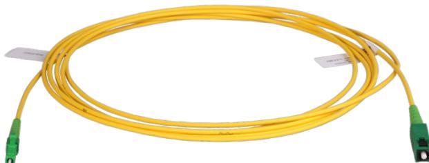
Master cables are selected assemblies with reference connectors on each side. They are used for repeatable IL/RL measurements of assemblies and links. The reference cables are defined in the following standards:
