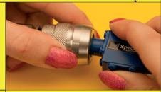
3. Push "Lock Nut" forward and engage the Push-On end of the Adapter with the mating female. Back nut must be released.
