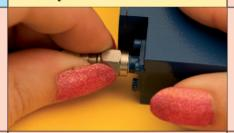
3. Just slide the Push-On SMA female Connector onto any standard SMA male. The connection is securely connected in seconds.
